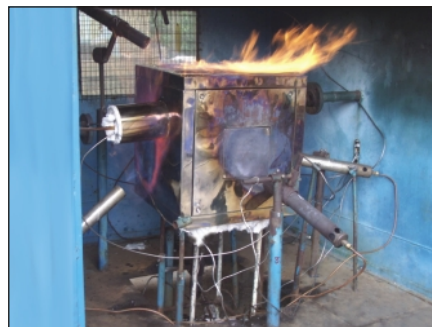
Fire Proof Enclosures Lloyds Certified. Protects actuator control systems against hydro-carbon fires.
