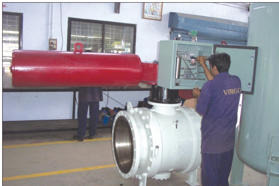
20" #150 FB Ball Valve with Pneumatic Spring Return Actuator for ESD service with Partial Stroking System
